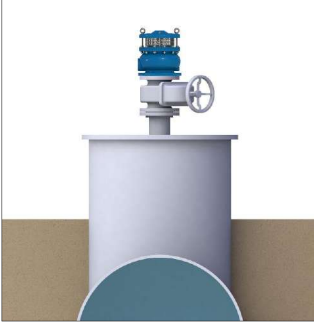
Single Vacuum Breaker on an Isolating Valve at 45° to Air Valve outlet
