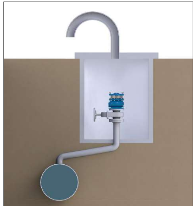
Two Vacuum Breakers on a shared Isolating Valve. The outlets face outward and the Isolating Valve at 45° to Air Valve outlets
