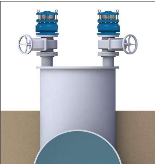
Two Vacuum Breakers on an Air Trap with separate Isolating Valves. The outlets face outward and the Isolating Valves at 45° to Air Valve outlets
