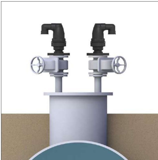
Two Air Valves on an Air Trap with separate Isolating Valves. Air Valve outlets face outward and the Isolating Valves at 45° to Air Valve outlets
