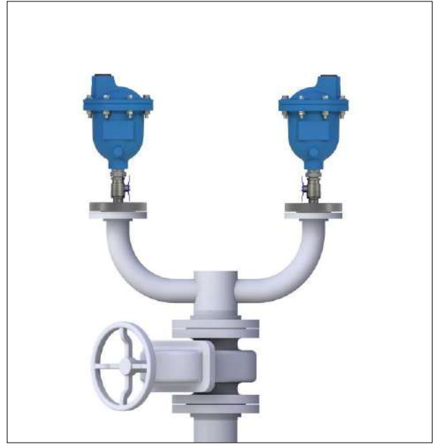
Two Air Valves on a shared Isolating Valve. Air Valves outlets face outward and the Isolating Valve at 45° to Air Valve outlets
