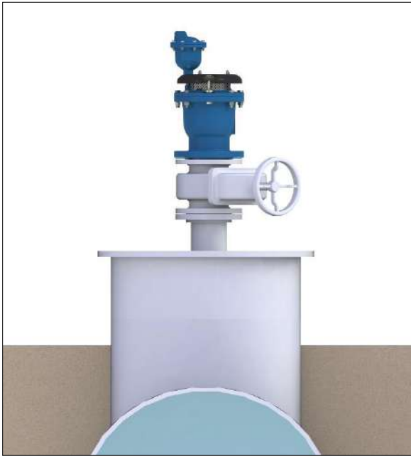
Single Air Valve on an Isolating Valve at 45° to Air Valve outlet
