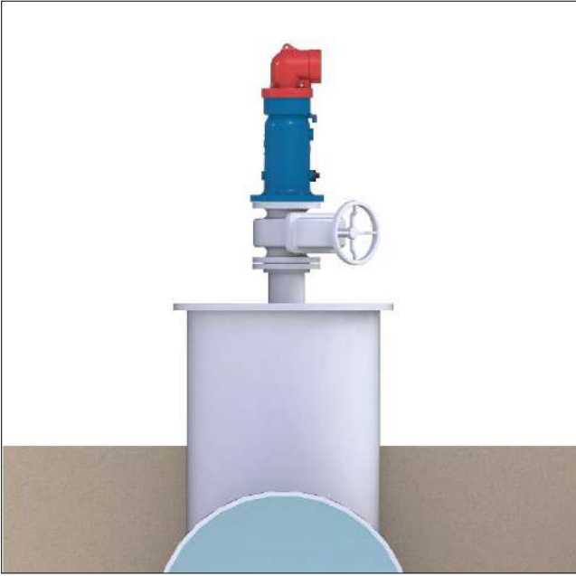
Single Air Valve on an Isolating Valve at 45° to Air Valve outlet
