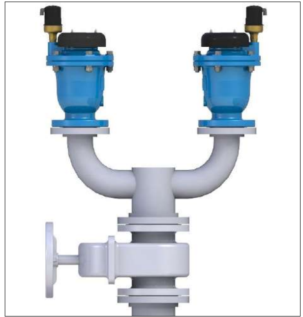
Two Air Valves on a shared Isolating Valve. Air Valves outlets face outward and the Isolating Valve at 45° to Air Valve outlets
