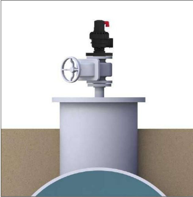
Single Air Valve on an Isolating Valve at 45° to Air Valve outlet
