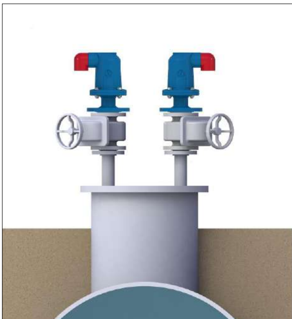
Two Air Valves on an Air Trap with separate Isolating Valves. Air Valve outlets face outward and the Isolating Valves at 45° to Air Valve outlets
